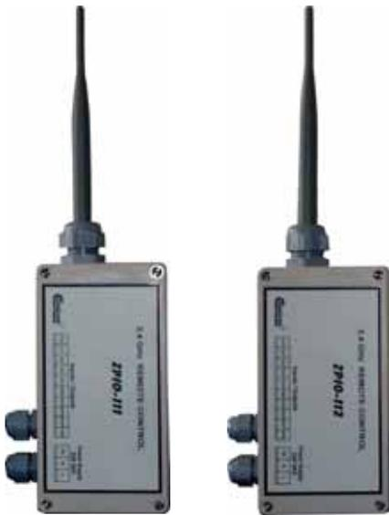
**ZPIO** modules replace the cable between the signal transmitter and the receiver with a reliable wireless connection. Data delivery between ZPIO modules is guaranteed by the applied protocol for transmission with confirmation, standard IEEE 802.15.4 and ZigBee.
